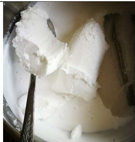
This paste (at 40:150 Pro-Tex 1405MS:Water) can be stored at room temperature for later applications in various products.
